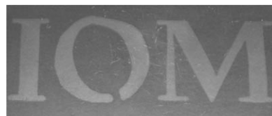
Figure 2. Poly( 4 ) coatings on glass prepared by the action of PI-1 .
